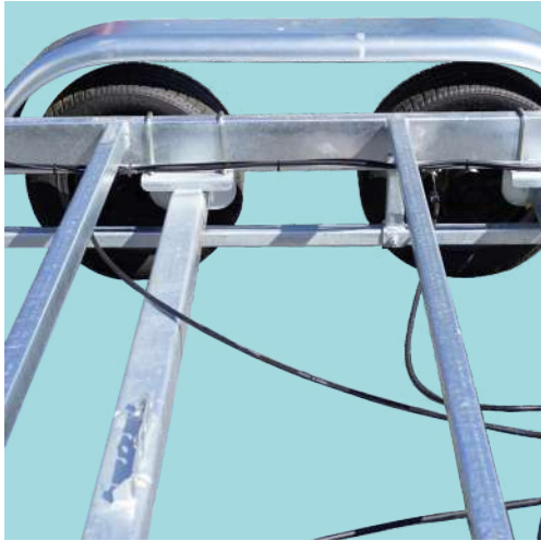
Fender bracket can be moved independently of the axle - free choice of fenders.
