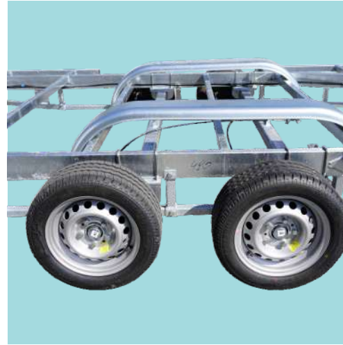
Adjustable axles to match the centre of gravity of the body. Plus a crossmember that allows you to mount the shock-absorber to the frame.
